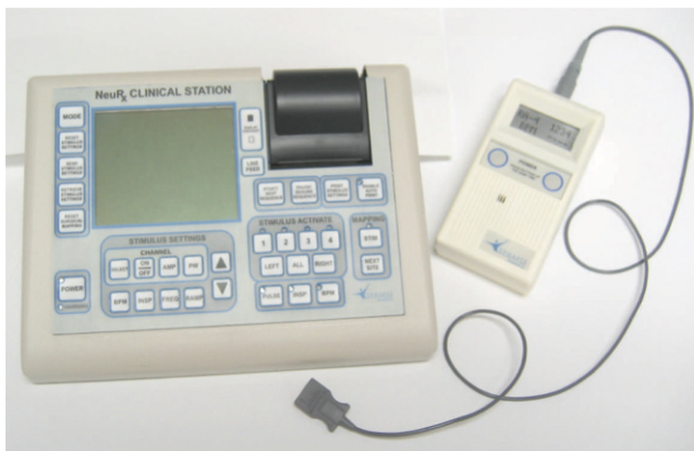
Figure 3 - The clinical station and the diaphragmatic pacing device.
