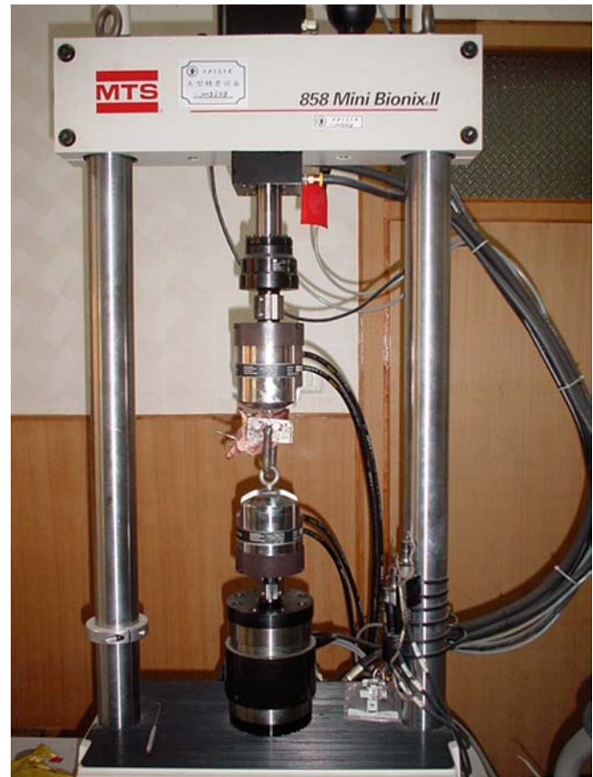
Fig. 2 Screw axial pullout test. The pull-out force is coaxial with the screw
