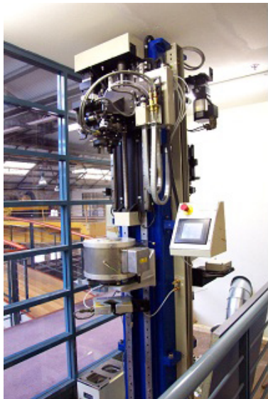
Figure 5. Top section of the fibre draw tower on the secondary side. Note in particular the chuck feed (top) and the furnace (middle), connected to the control unit (right).
