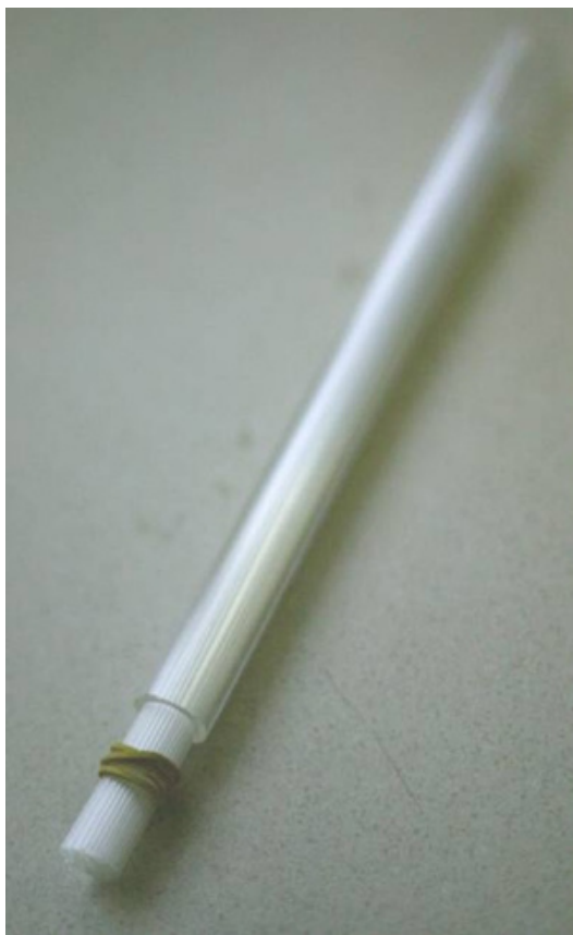
Figure 12. Inserting indium wire stacked bundle into PMMA tube.
