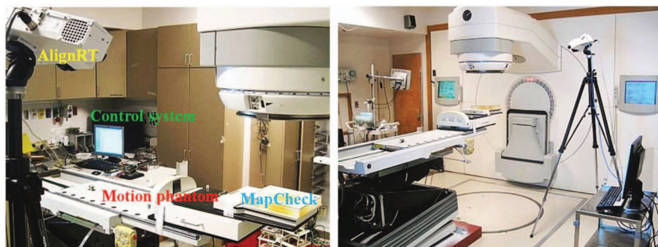
FIG. 7. Experimental setup of the tumor motion compensation system.
