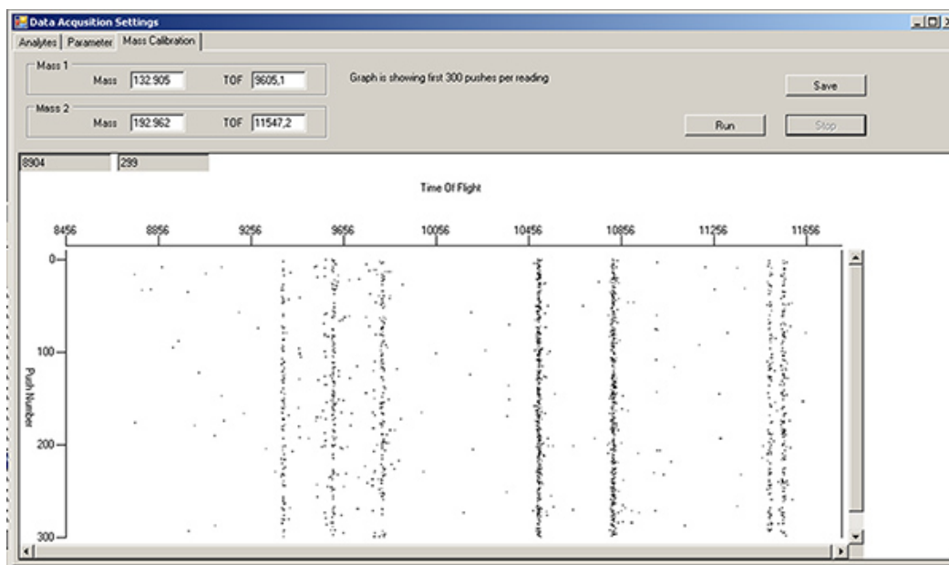
Figure 4. Mass calibration tab window, showing vertical streaks for various isotopes in DVS tuning solution. Click here to view larger figure.
