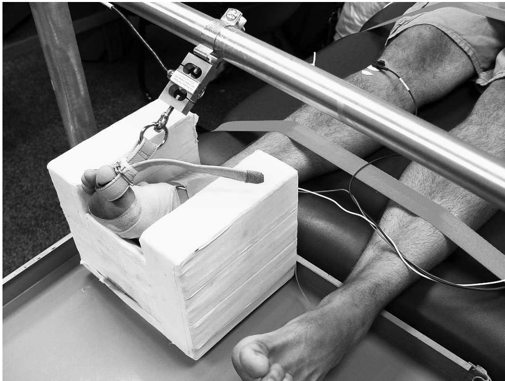
Figure. Great toe harness and strain gauge attachment.
