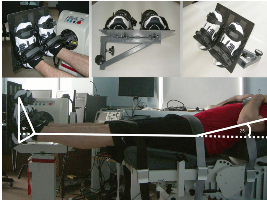
Figure 5 Experimental setup. Initial position for the MVCs and the fatiguing exercises. Also depicted is the custom attachment which allowed the simultaneous assessment of both ankles on the Biodex System 3.
