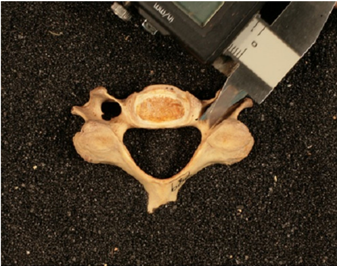
Fig. 3 Pedicle length as measured from superior aspect of the cervical vertebrae. The average of both pedicles was used in the study
