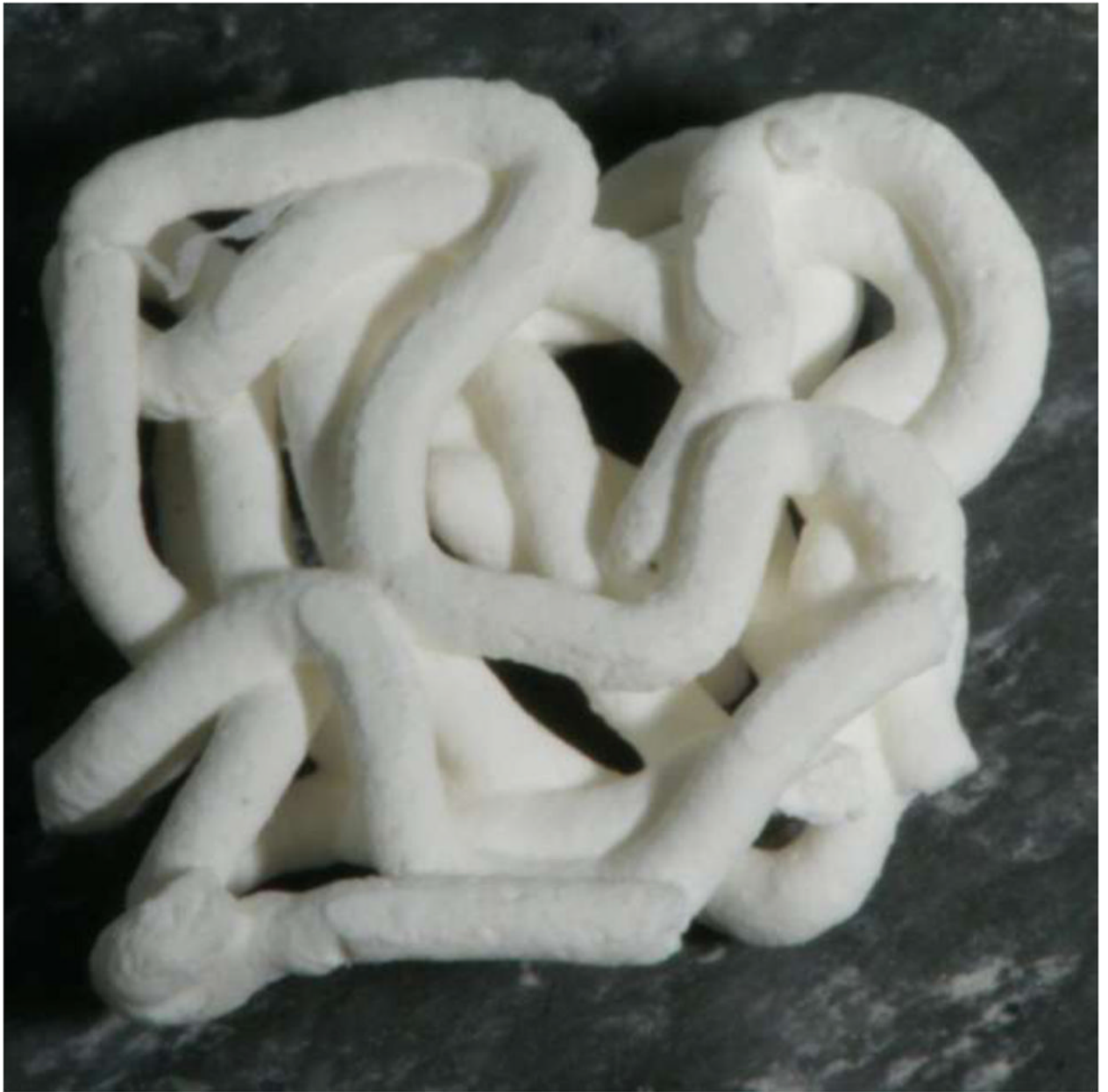
Fig. 1. GEMOSIL paste for direct scaffolding. Formable GEMOSIL paste can be molded into a (a) cube by hand and injected to form a (b) porous scaffold
