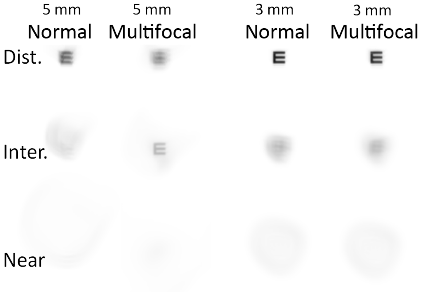
Figure 9. Simulated vision for a normal wavefront profile and a normal profile with added spherical aberration ( -0.274 \mu\text{m} for 5.0 mm pupil). 20/20 Snellen E letter (0 logMAR) was convolved with point-spread function with 0.00, -1.00 D, and -2.50 D of defocus (Dist. = distance; Inter. = intermediate).
