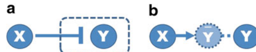
FIG. 2. (a) Inhibition edge ( X inhibits Y ), and (b) modified edge ( X activates \bar{Y} and the relation between \bar{Y} and Y is defined by Boolean logic or algebraic constraint).
