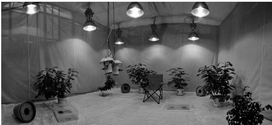
FIGURE 1. Interior of one mesocosm, showing resting pots, oviposition sites, lights, temperature and humidity sensors, a chair for the blood host, and nectariferous plants.
