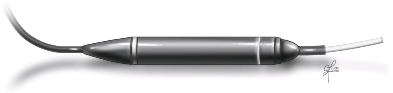
Figure 3. The 3×3 curved array ultrasound probe used in this study. The size of the probe is approximately that of a No. 5 Frazier suction.
