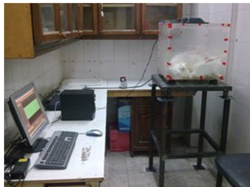
Figure. 1: A cross-sectional view of exposure chamber (50×50×50 cm polycarbonate Plexiglas) has been shown. All rabbits were located into this chamber for exposure to noise pollutant (N group) and control group for 8 hr per day during 5 consecutive days. Exposure to noise has been carried out through a noise loudspeaker mounted on the roof of the chamber. Control group is just posed onto the chamber resembled to other groups with identical situations, but without any exposure.
