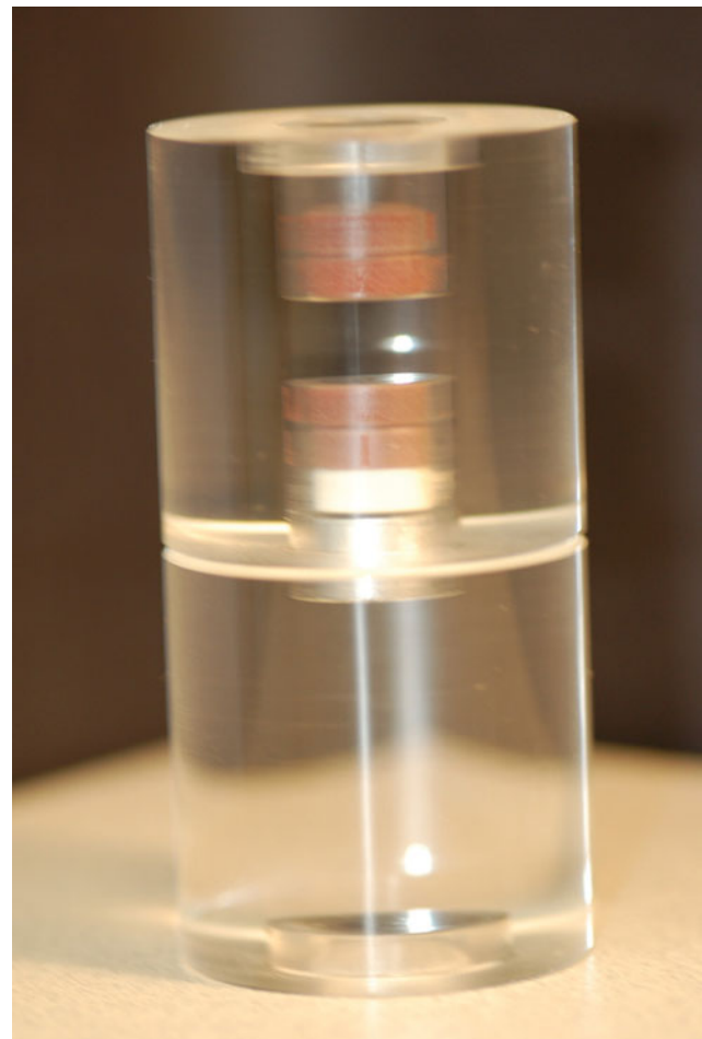
Figure 1 Three-dimensional eight-tissue radiographic phantom
