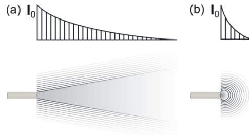
Fig. 11. Schematic of different shape of absorption volume and possible shape of pressure sources for (a) \mu < 5.5 \text{ cm}^{-1} and V \gg 1 and (b) \mu > 5.5 \text{ cm}^{-1} and V \ll 1 .
