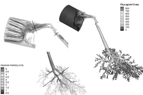
FIG. 3. Regional airflow velocities (m/s) in the nose, larynx, and lung and corresponding acrolein flux rates (pg/cm 2 /s) of the monkey CFD/PBPK model. Steady-state CFD simulations were conducted at twice the resting minute volume (907 ml/min) and a constant inhalation concentration of 0.6 ppm acrolein in the cylinder. Solid black lines in the CFD simulations indicate cross sections of the nose, mouth, larynx, and lung regions used to calculate the Reynolds numbers in Table 5.
