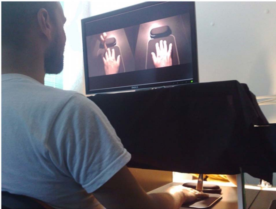
Figure 2. The video-mediated system as used for the advART condition. In this (advART) as well as in the other two condition the participant sits in front of the system and observes the mirrored images of his hand(s) either on the screen or in the optical mirror while an assistant is brushing the participant's right hand. In the advART condition, shown in this picture, the participant sees the mirror image of his actually brushed right hand on the left side of the screen while the mirror image of his left hand is shown on the right side of the screen. doi:10.1371/journal.pone.0050942.g002
