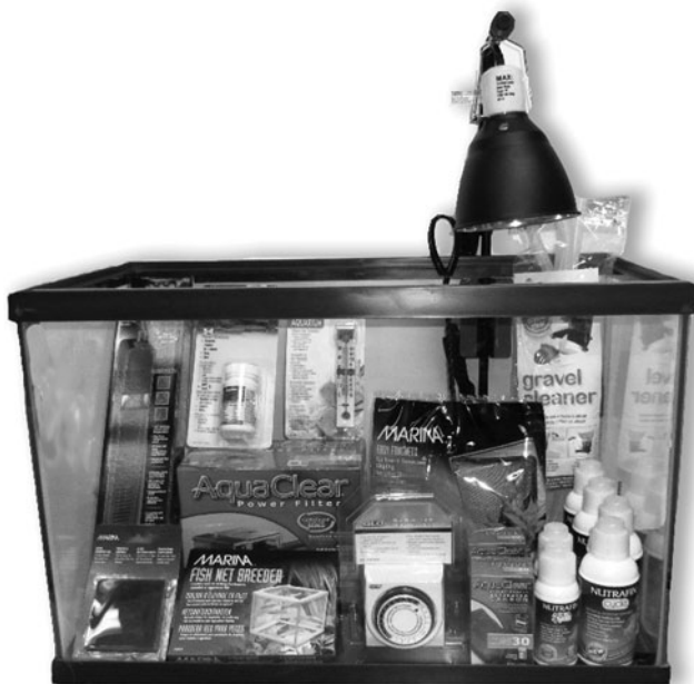
FIG. 1. The tanks used for these experiments included: Deep Sea Aquatics (Ocean View 20 High or 29), AquaClear 30/50 filter A600/10, Hagen Fluval 200/300 Watt Heater HE-A784/5, AquaClear Carbon 30/50 A602/12, Marina 3," 8" Nets A1273/77, Glo Dual Timer A3890, Nutrifin Cycle, 8 oz. A7610, 20- and 29-gallon fish tanks, Repti Glo 5.0 Light Bulb PT2186, clip-on lamp fixture, and Marina Gravel Cleaner A1062.
