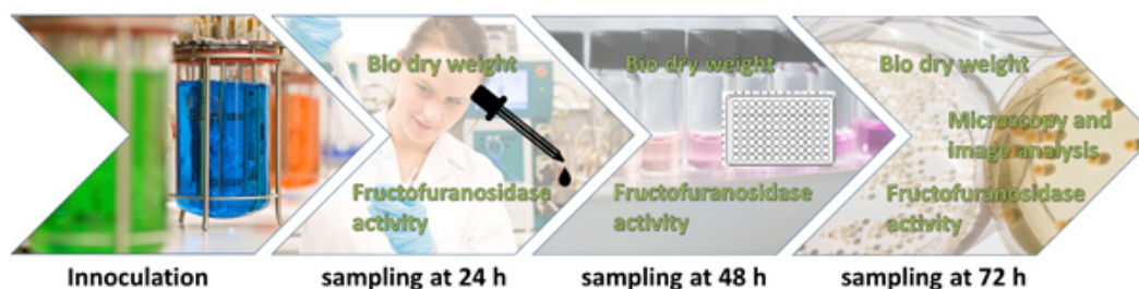
Figure 1. Overall scheme of the experimental design and the analytic procedure. A. niger is cultivated (with or without micro particles) in a 3 L stirred tank bioreactor for 72 h. After 24, 48 and 72 h a sample is taken for determination of biomass dry weight and β-fructofuranosidase activity, which again are used for calculation of the specific productivity. After 48 h the fungal morphology is examined by microscope and characterized by digital image analysis. Relevant parameters of image analysis are combined to a Morphology number, which is mathematical correlated with the specific productivity.
