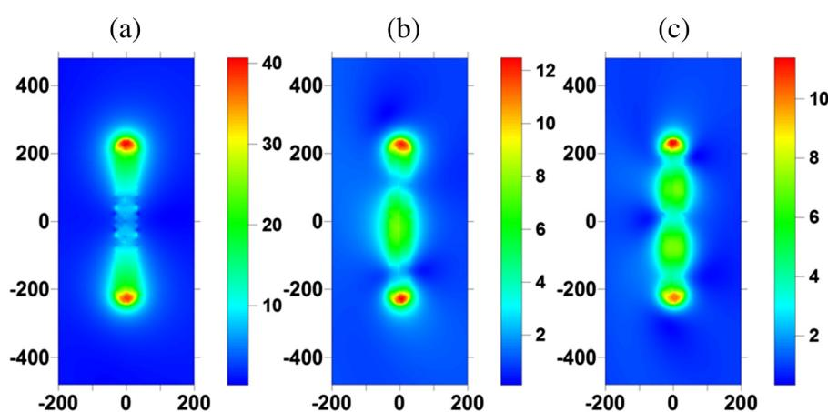
**Figure 3** Electric field distributions at the first, second, and third modes of GNR. Electric field distributions at the (a) first (dipole, 1,870 nm), (b) second (quadrupole, 960 nm) and (c) third (sextupole, 700 nm) modes of GNR ( $a = 30$  nm, AR = 8) irradiated by an obliquely incident plane wave of  $\theta = 15^\circ$ .
