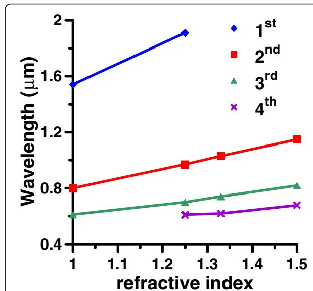
**Figure 8** Wavelengths of the first, second, third and fourth modes of GNR versus refractive index. Wavelengths of the first, second, third and fourth modes of GNR ( $a = 30$  nm) versus refractive index ( $n = 1$  to  $1.5$ ) of medium for  $AR = 8$ .
