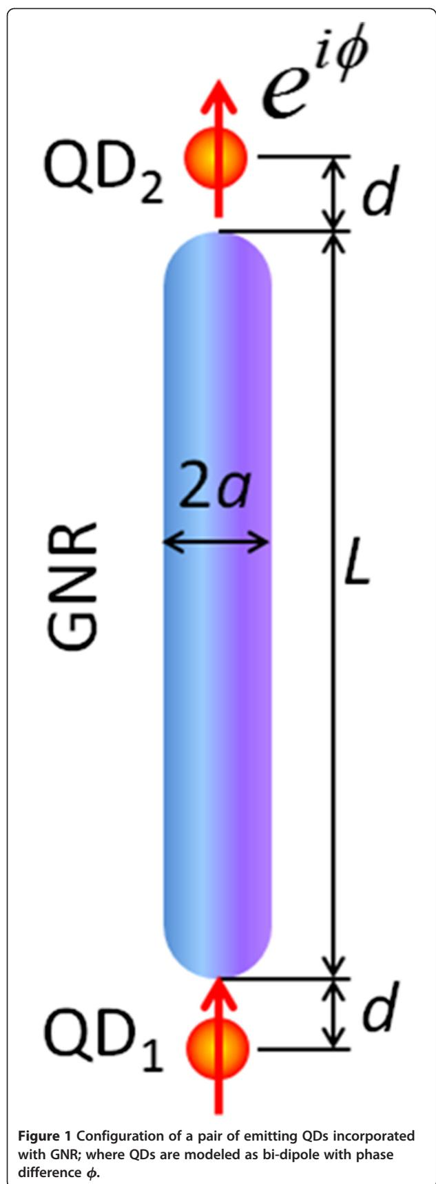
**Figure 1** Configuration of a pair of emitting QDs incorporated with GNR; where QDs are modeled as bi-dipole with phase difference  $\phi$ .
