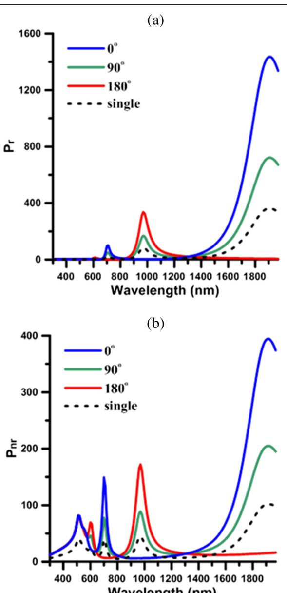
**Figure 4** Radiative power and nonradiative power of bi-dipole with phase difference. (a) Radiative power and (b) nonradiative power of bi-dipole with phase difference ( $\phi = 0^\circ, 90^\circ, 180^\circ$ ),  $a = 30$  nm, AR = 8,  $d = 15$  nm. Dashed line, single dipole.
