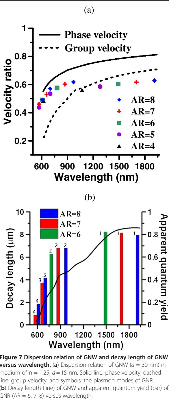
**Figure 7** Dispersion relation of GNW and decay length of GNW versus wavelength. (a) Dispersion relation of GNW ( $a = 30$  nm) in medium of  $n = 1.25$ ,  $d = 15$  nm. Solid line: phase velocity, dashed line: group velocity, and symbols: the plasmon modes of GNR. (b) Decay length (line) of GNW and apparent quantum yield (bar) of GNR ( $AR = 6, 7, 8$ ) versus wavelength.
