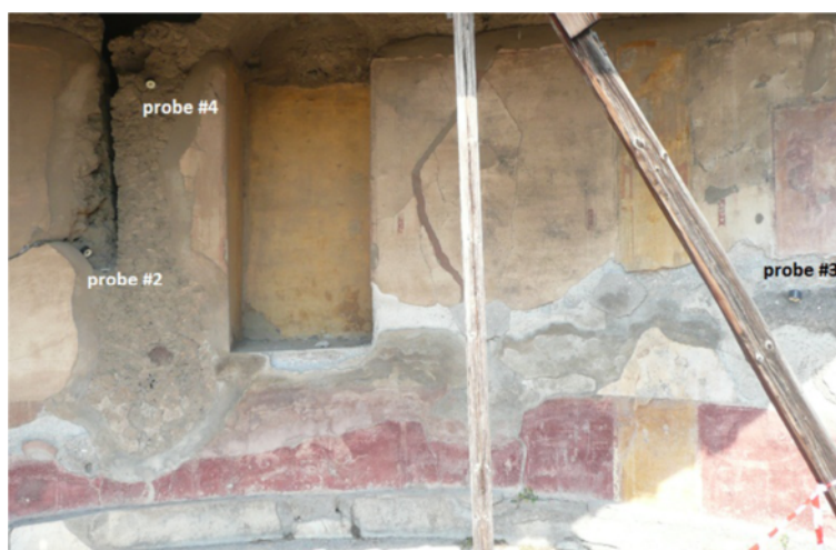
Figure 6 Location of probes #2, #3 and #4 in room 4. The picture was taken at 1:05 PM. The brighter zone at the lower right corner corresponds to sunlight incident on the frescoes that affects #3 from 2:00 PM to 8:00 PM.
