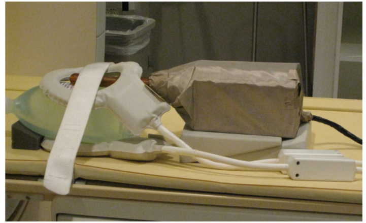
Fig. 7. Experimental setup for SNR tests in a 3 T MRI scanner. Left image shows unshielded robot, saline phantom, and imaging coils. Right image shows the robot with the addition of radio-frequency (RF) shielding.
