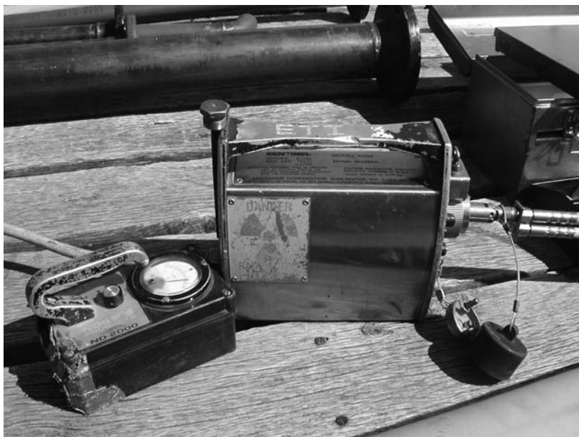
Figure 1. Iridium-192 Isotope Camera [Reprinted with permission by Larry R. Ewer, C.W.I., President, ETI Ewer Testing and Inspection, Inc. www.etitesting.com ]
