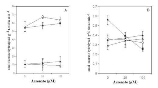
**Fig. 2.** Effect of arsenate  $(Na_2HAsO_4.7H_2O)$  and phosphate  $(KH_2PO_4)$  applied either singly or in combination on the activities of sucrose synthase (SS) [A] and acid invertase [B] of ten days old rice (cv. MTU 1010) seedlings. Each data point expressed as the mean  $\pm$  SE (n=5).  $\blacksquare$ - As (Root);  $\triangle$ - As (Shoot);  $\square$ - As+PO<sub>4</sub> (Root);  $\triangle$ - As+PO<sub>4</sub> (Shoot).
