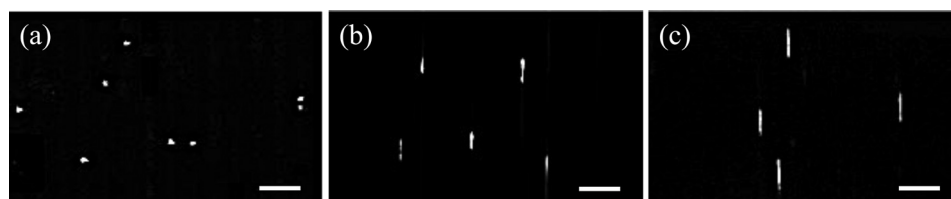
FIG. 7. Representative fluorescent micrographs showing \lambda -phage DNA strands in cylindrical glass nanocapillaries with a diameter (a) \text{\O}400 nm, (b) \text{\O}200 nm, and (c) \text{\O}50 nm, fabricated in silicon trenches with a depth of 2.5 \mu\text{m} and a width of 2.5 \mu\text{m} in (a) and 3 \mu\text{m} in (b) and (c). Scale bars: 20 \mu\text{m} .
