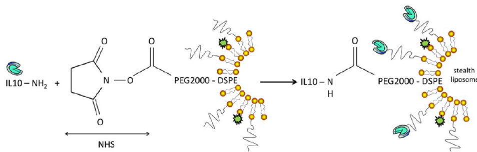
Figure 1. Coupling reaction of IL-10 to liposomes. Recombinant IL-10 was coupled to PEGylated stealth liposomes via amine-reactive carboxylic acid succinimidyl (NHS) ester binding. The unbound protein was removed by dialysis.
