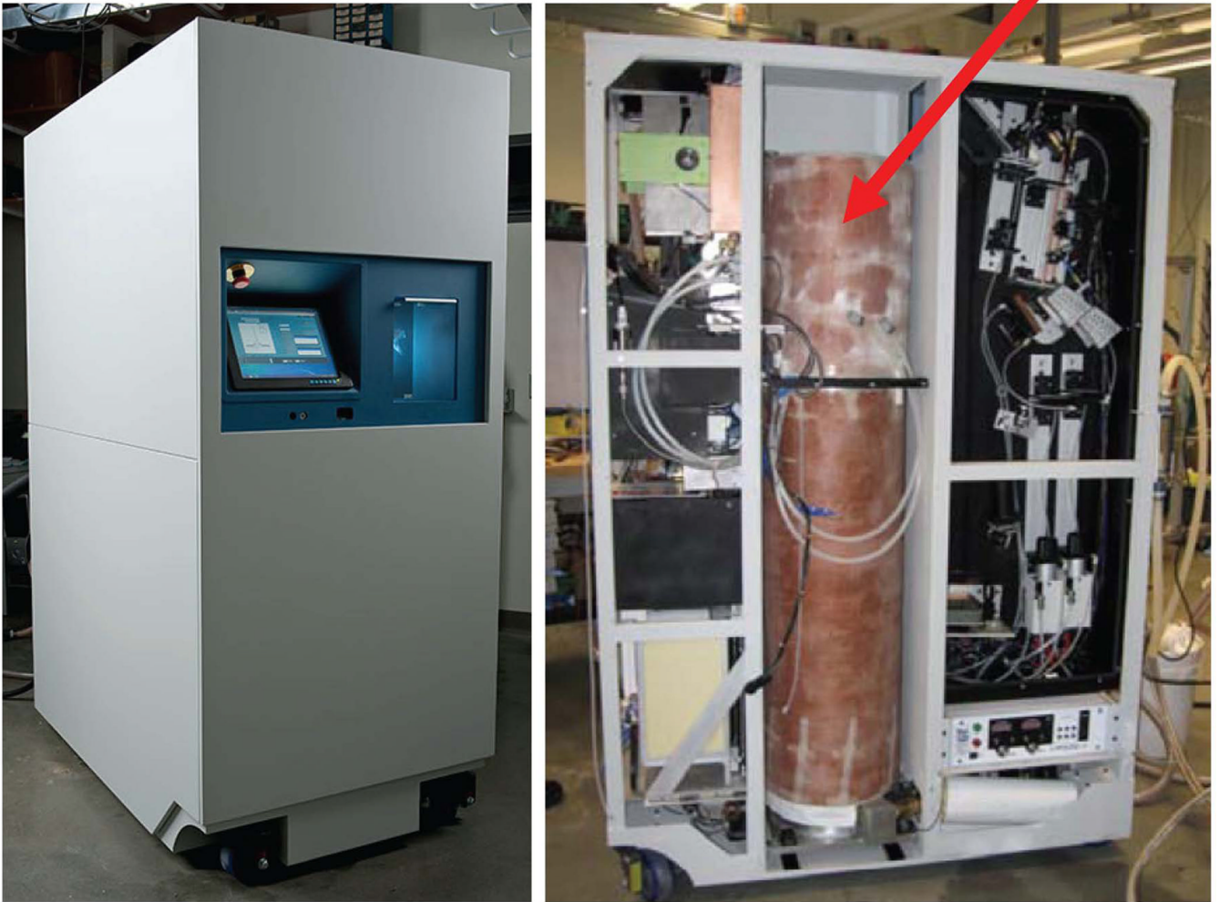
Figure 2. State-of-the-art gas-polarization system for ^{129}\text{Xe} . These photographs show a prototype commercial fourth-generation gas-polarization system optimized for ^{129}\text{Xe} (model XeBox-E10, Xemed, LLC, Durham, NH). This polarizer is based on the flowing approach for hyperpolarized-gas production as discussed in the text. The polarizing column, which is the functional analog of the optical cell shown in Fig. 1, is indicated on the right. Additional technical details can be found in ref. (28).
