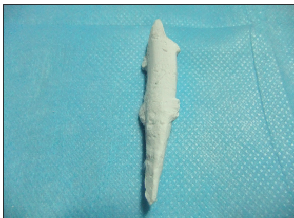
Figure 1. Chitosan fiber/calcium phosphate ceramics composite scaffold.
