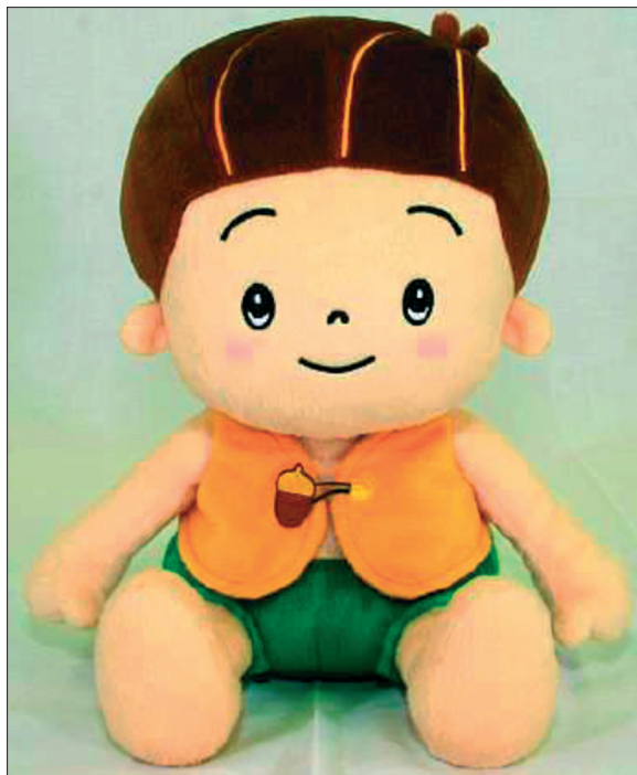
Figure 2. Photograph of a communication or control robot. The robot is 28 cm in height and 680 g in weight. The features of shape, voice, and motion resemble those of a 3-year-old boy. The robot was programmed to behave as if communicating with customers and to release affective behavior that could develop a friendly relationship, in particular with elderly people. The control robot has the same shape as the communication robot, however, the control robot was not constructed to talk or nod to the participants.
