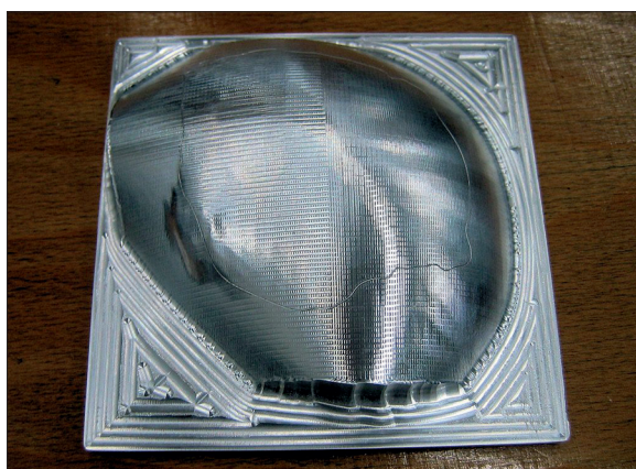
Figure 7. Material form produced using Rapid Prototyping to profile the prosthesis by a manufacturer – Case B.
