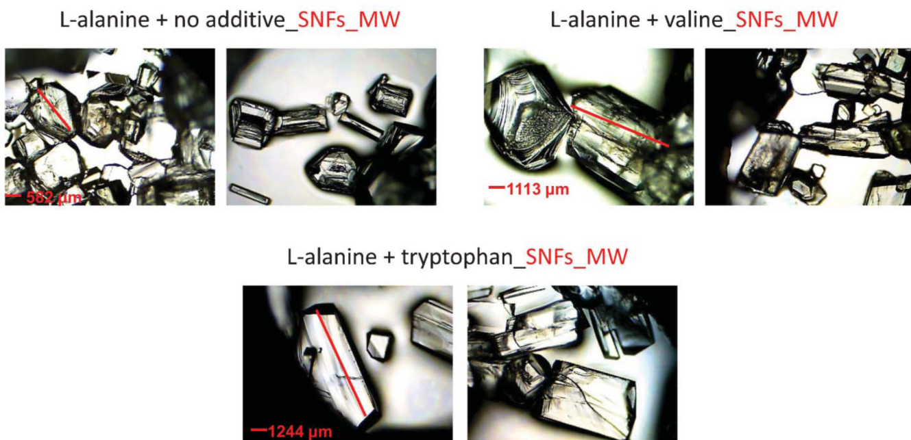
Fig. 5. Comparison between L-alanine (no additive), L-alanine with valine, and L-alanine with tryptophan using MA-MAEC.
