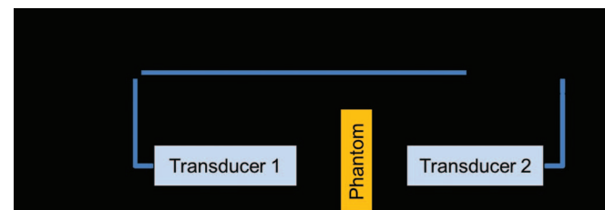
FIG. 4. Schematic diagram used for the measurement of acoustic properties of tissue mimicking materials.
