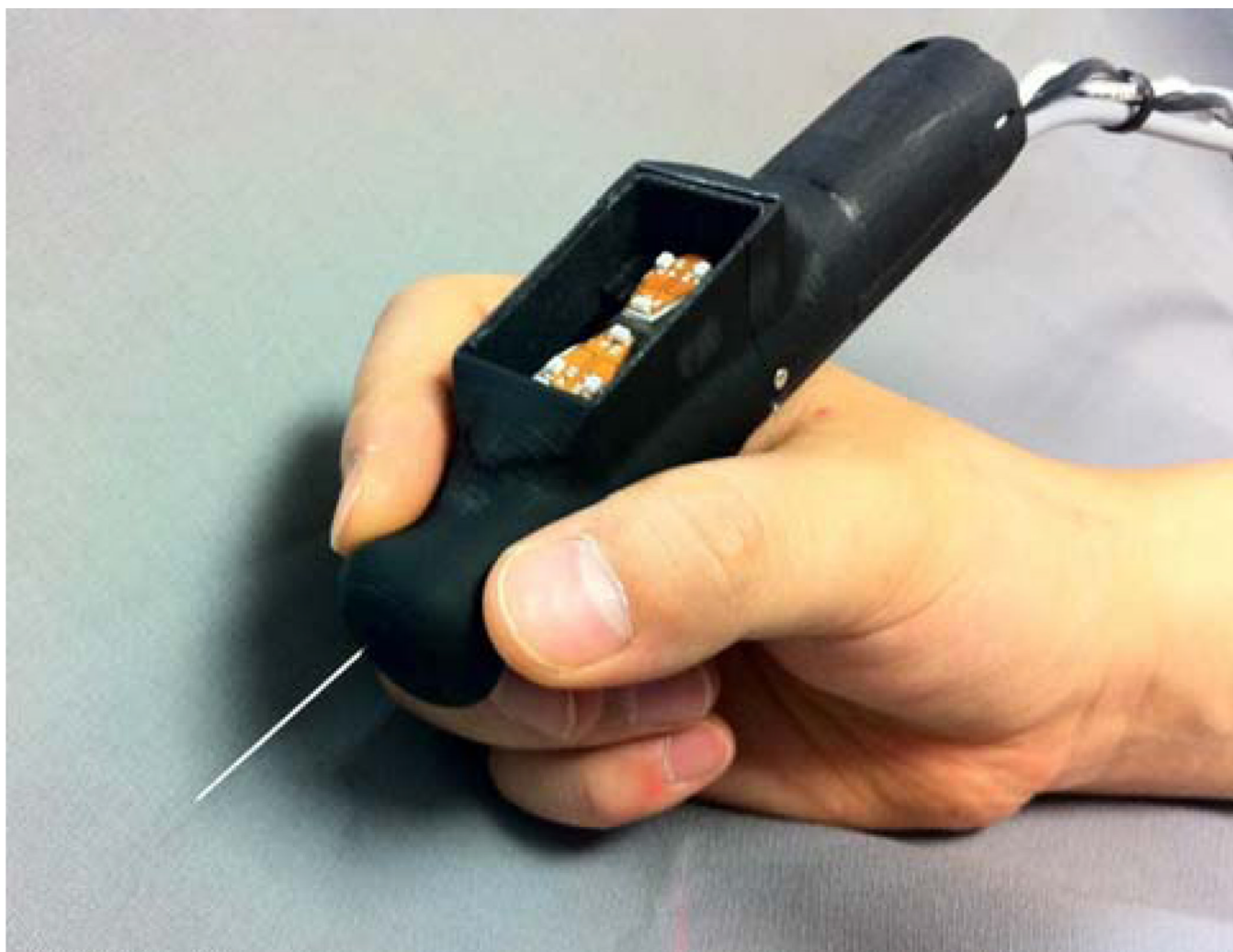
Figure 1. Micron, an active handheld micromanipulator.
