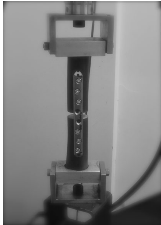
Fig. 2 An open sample undergoing fatigue testing is shown.
