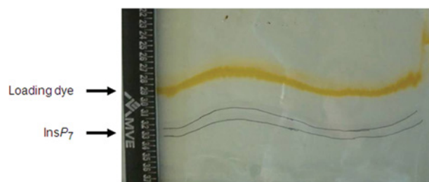
Figure S2 Dye-front guided excision of PP-InsP
