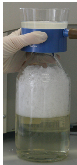
FIGURE 2. Formation of foam in culture supernatants of T. atroviride upon filtration. Processing of the culture filtrate of T. atroviride after growth conditions that were used for production of large amounts of native EPL1 showed excessive foaming upon filtration and ultrafiltration steps.
