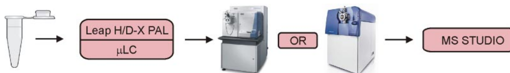
FIG. 1. Configuration of HDX-MS platforms for comparing MS performance in peptide sequence mapping, deuteration precision, and accuracy. Sample digests (deuterated or undeuterated) were introduced into either an Orbitrap Velos or a 5600 TripleTOF using matched gradient microLC systems, to ensure that peptide retention times were equivalent. Mass Spec Studio was used for deuteration analysis.
