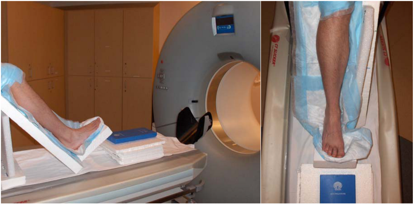
Figure 1. Position and orientation of lower extremity sample in Styrofoam fixture during vQCT scanning. Hydroxyapatite calibration phantom is shown in front of the foot, at the height of the talus.
