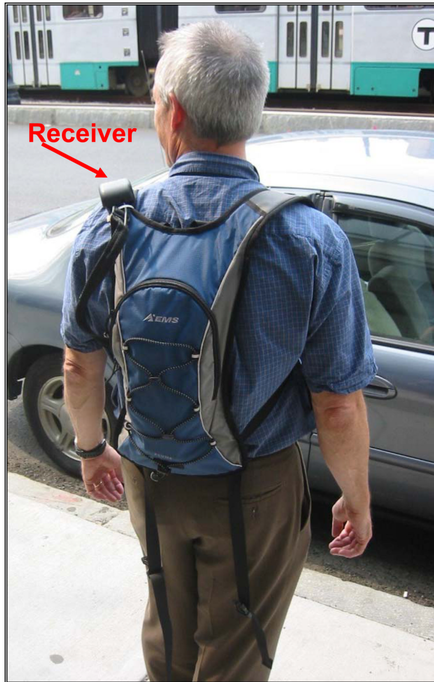
Figure 1. GPS unit with receiver on shoulder strap.
