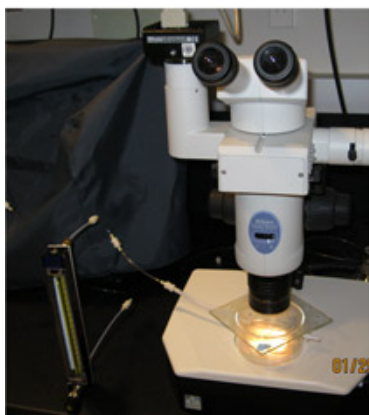
Figure 3. Visualization of C. elegans in hypoxia with microscopy. Worms are exposed to hypoxia using the methods outlined. The transparent environmental chamber (constructed with a pyrex crystallization dish and glass plate) is placed directly on the stage of a dissecting scope. Two views are shown, one including the entire gas flow set up, the other with just the chamber on the microscope stage.
