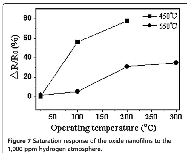
**Figure 7** Saturation response of the oxide nanofilms to the 1,000 ppm hydrogen atmosphere.
