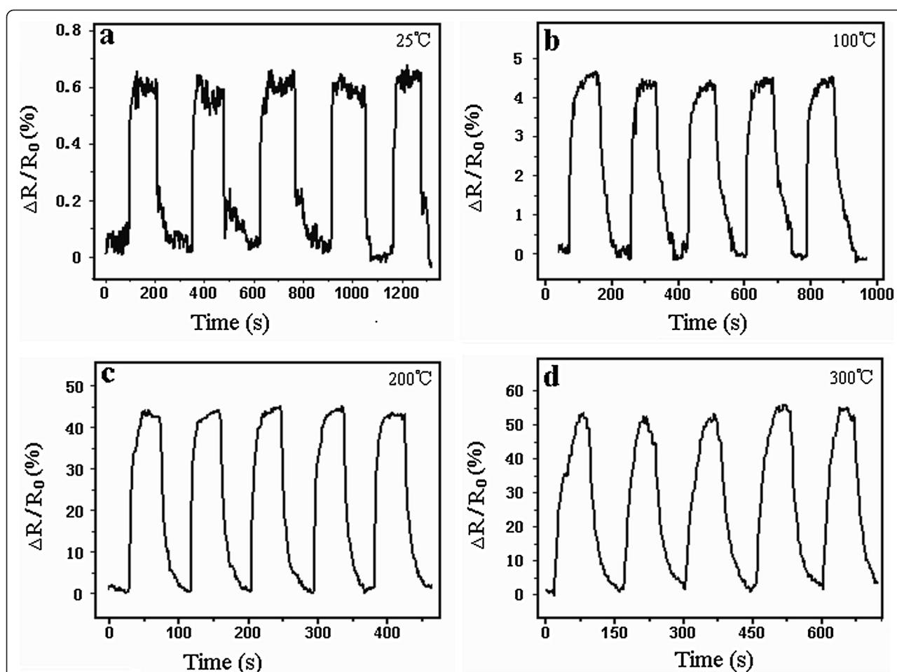
**Figure 6** Response curves of oxide nanofilms annealed at 550°C. The operating temperatures were (a) 25°C, (b) 100°C, (c) 200°C, and (d) 300°C.
