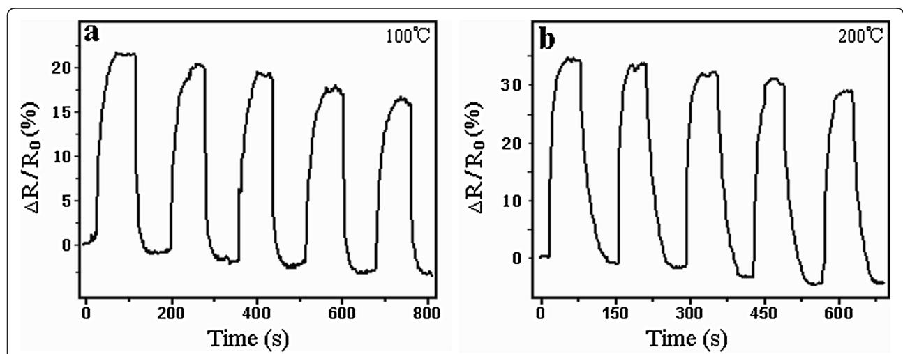
Figure 5 Response curves of oxide nanofilms annealed at 450°C. The operating temperatures were (a) 100°C and (b) 200°C.
