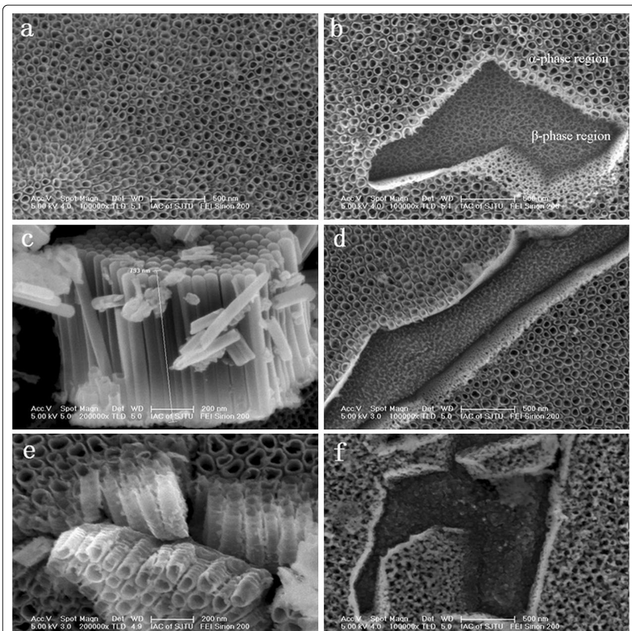
**Figure 2** SEM images of the oxide nanofilms before and after annealing. (a) Top view of as-anodized sample, (b) α- and β-phase regions of as-anodized sample, (c) cross-sectional view of the Ti-A-V-O nanotubes, (d) top view of oxide nanofilms annealed at 450°C, (e) cross-sectional view of oxide nanofilms annealed at 450°C, and (f) top view of oxide nanofilms annealed at 550°C.
