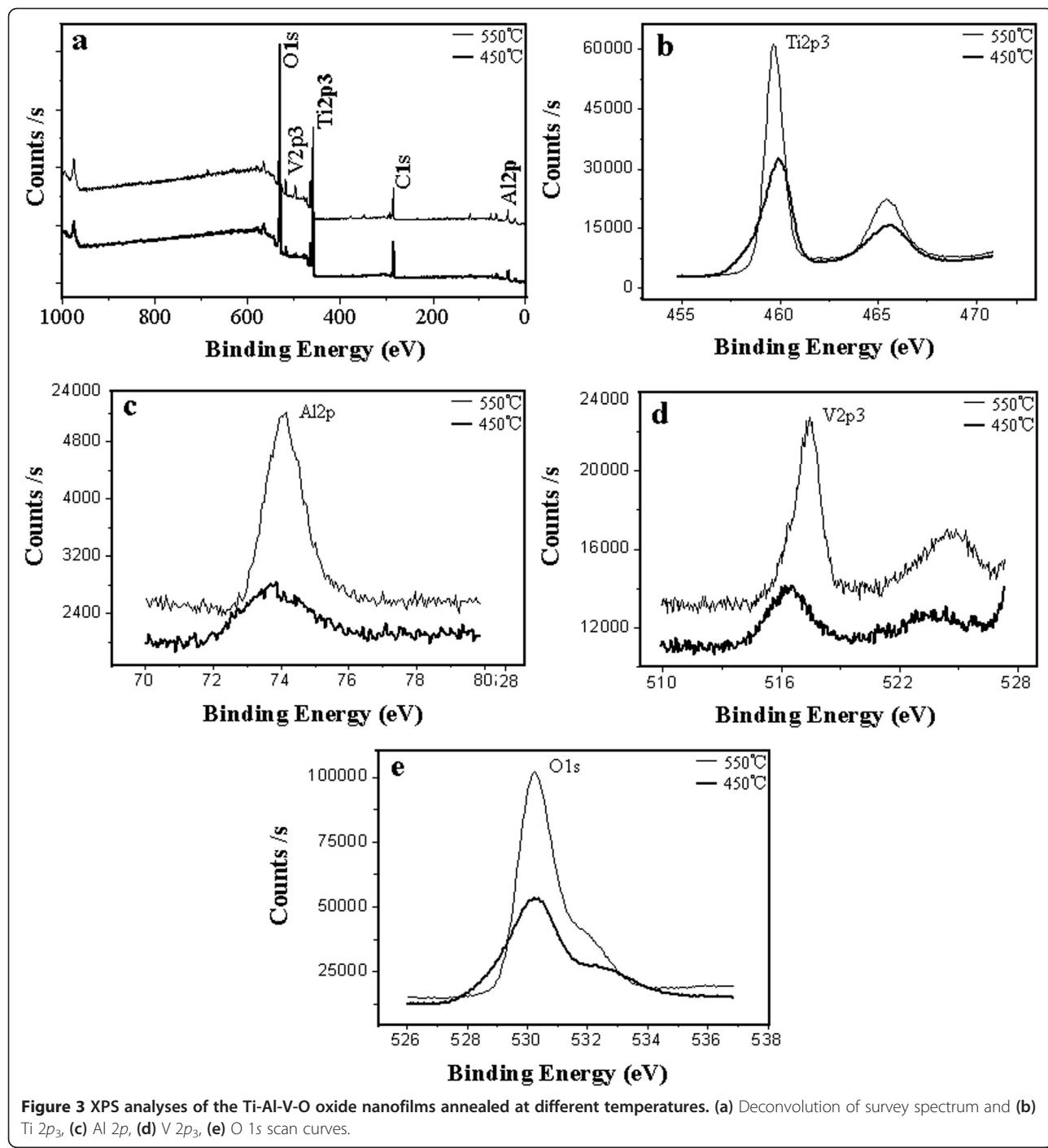
**Figure 3** XPS analyses of the Ti-Al-V-O oxide nanofilms annealed at different temperatures. (a) Deconvolution of survey spectrum and (b) Ti 2p<sub>3</sub>, (c) Al 2p, (d) V 2p<sub>3</sub>, (e) O 1s scan curves.
