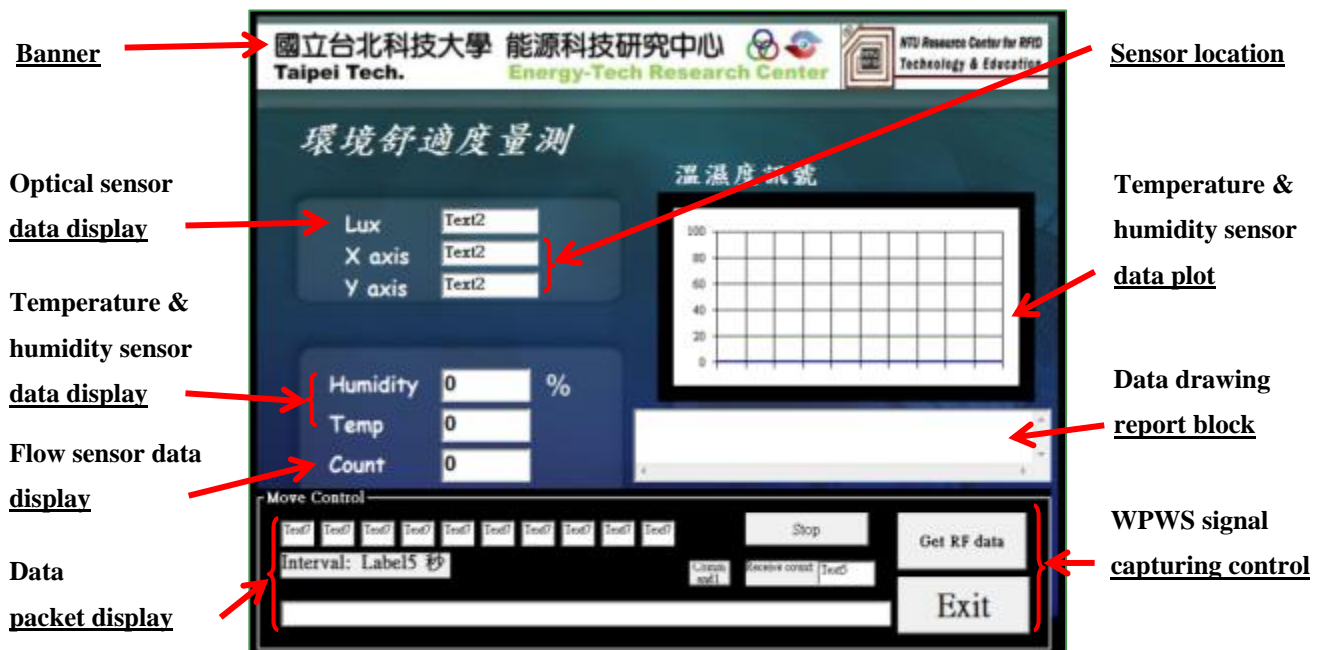
Figure 12. The software used to display sensing data, record communication packets, and evaluate the stability of the WPWS.
