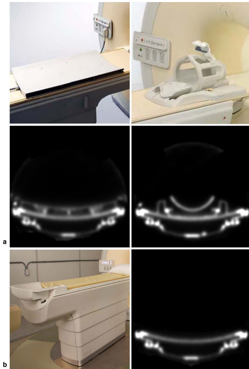
Fig. 6 In PET/MR, coils and other MR devices not visible in the MR images must be generated as template images, for example, in PET transmission scans and added to the attenuation map. Examples of a
