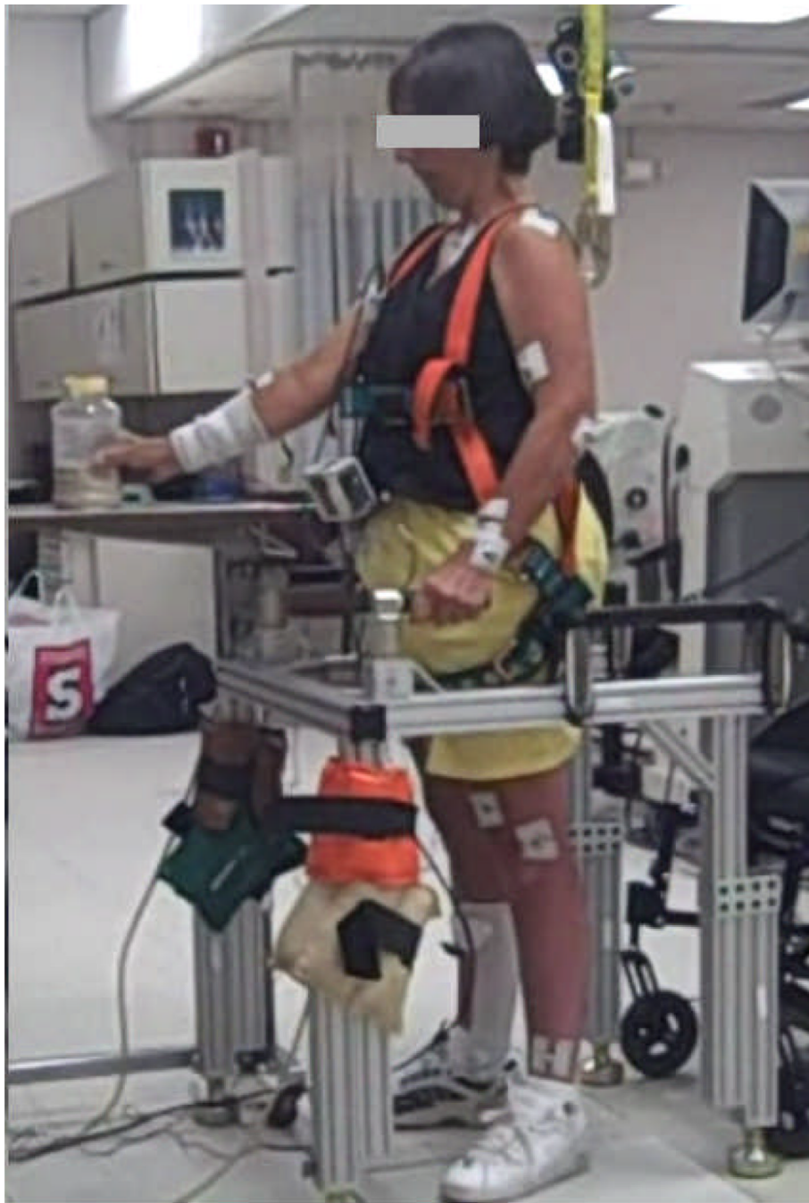
Figure 2. SCI subject undergoing internal perturbations by volitionally moving object over level surface with one arm while stabilizing with other arm.
