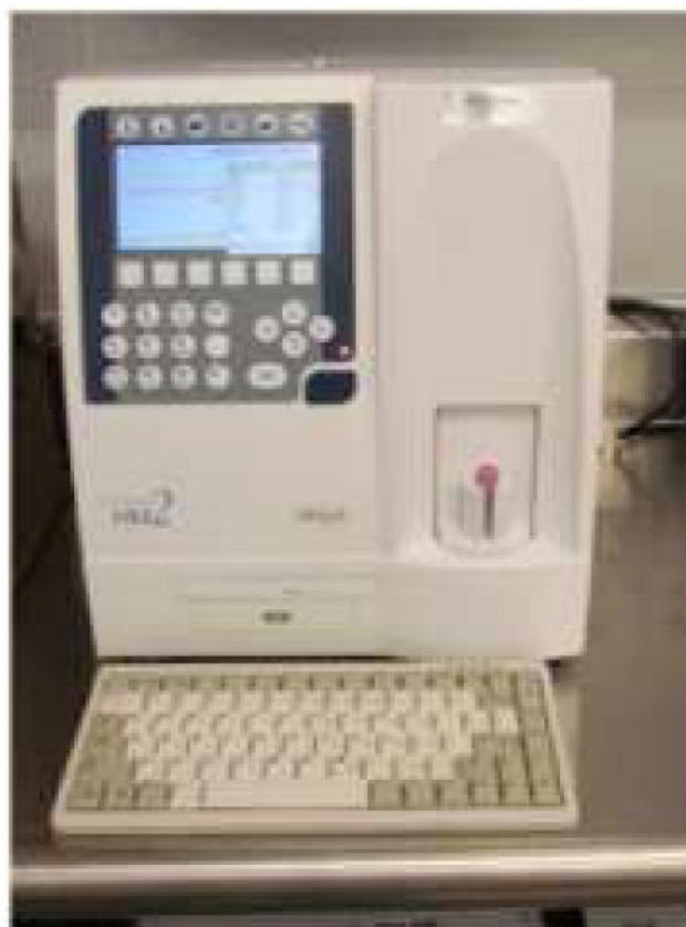
Figure 1. VetScan HM2 Hematology system (Curtsey: Abaxis Inc., Union city, CA)
