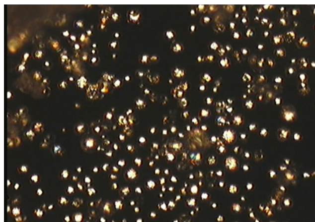
Fig. 4 Photograph of microcapsules of n -eicosane coated with polysiloxane taken by optical microscope with the illumination of sample by polarized light and observation with cross-polarization
