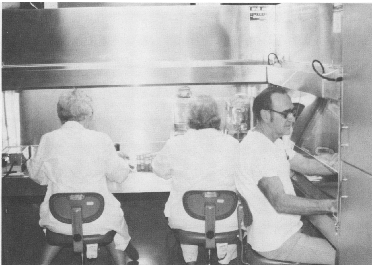
FIG. 12. Specialized class II cabinetry. Two cabinets are connected by a transfer cabinet to contain infectious microorganisms.
