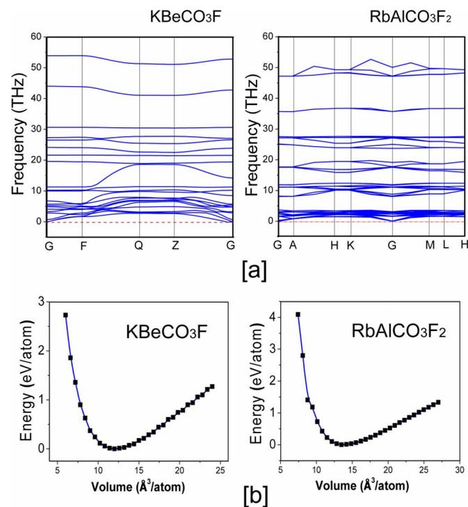
**Figure 2** | Evidences of the structural stabilities in  $\text{KBeCO}_3\text{F}$  and  $\text{RbAlCO}_3\text{F}_2$  from the first-principles studies. (a) The phonon spectra. (b) The total energy as a function of volume per atom. The energy minimum is set as the zero point.
