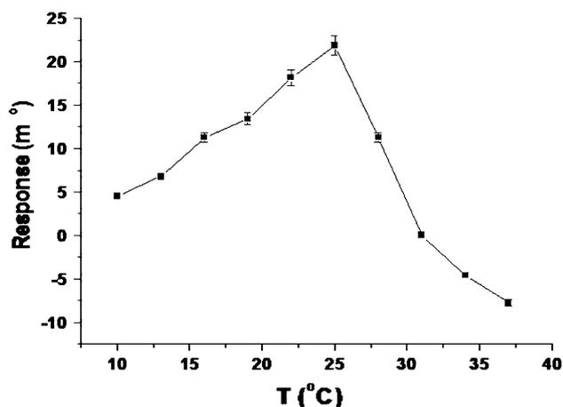
**Fig. 3** Graph showing SPR angle shift with temperature
