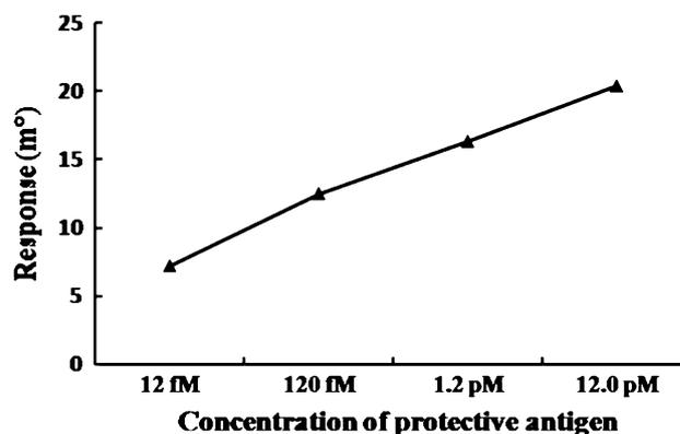
**Fig. 5** Calibration plot of SPR signal v/s various concentrations of PA a 12 fM; b 120 fM; c 1.2 pM; d 12 pM
